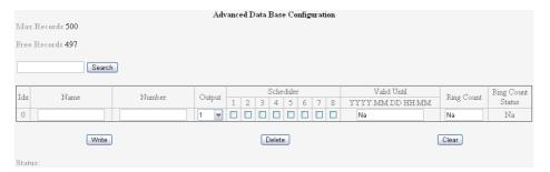
To add a new user using this menu section, fill in the information and press **Write** button. Each user information column is described below.
